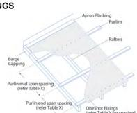
Use **Noise Stop Tape** on all battens, purlins or noggings to minimise the noises associated with expansion and contraction.
