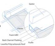
sheet through the crests for roofing and through the valleys for walls. Use 55mm fixings for Sunline corrugate profile polycarbonate roofing. For **roof laying**, start with the lower sheets first, keeping side laps away from prevailing wind. Allow an overhang of 50mm.
